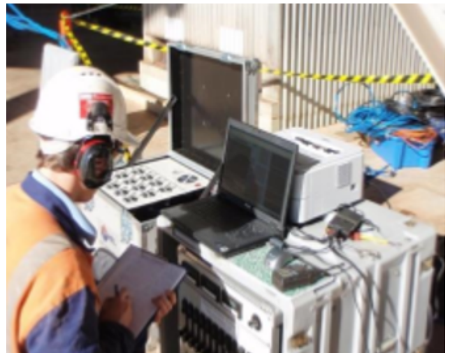
MCDA equipment in use determining combustion gas concentration profiles at a power station
