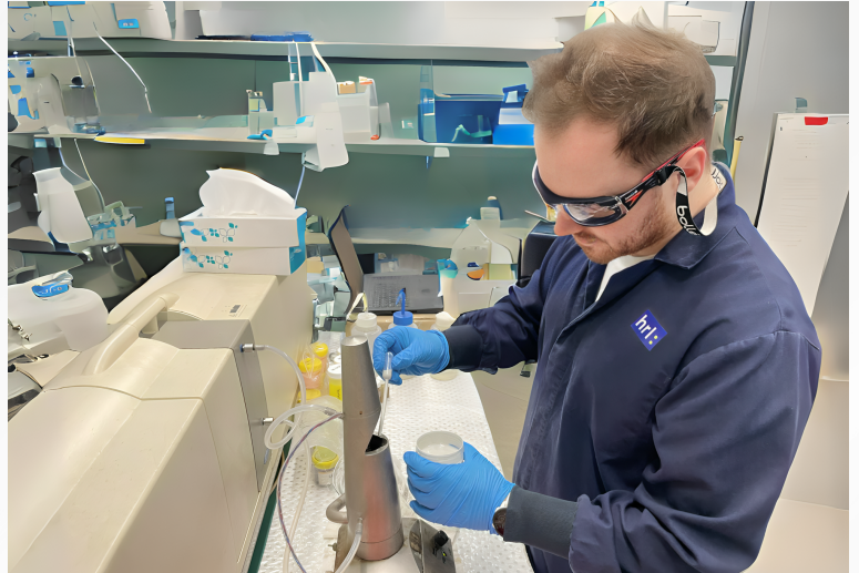
Callum analysing a chemical dispersion sample for laser particle size
